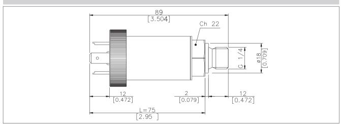
**Dimensions:** TKDA, due to the autozero & span board, is 5 mm (0.197 in) longer, so dimension "L" on TK data sheet
