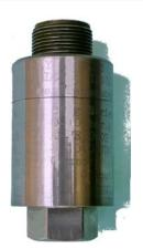
"AJAY SENSORS" Pressure Transducer, Type 201 - g series employs Strain Gauge (Foil Type) bonded to an integrally machined diaphragm and connected in a four active arm wheat stone bridge circuit. These transducers are fully temperature compensated for zero and sensitivity drift for a wide range.
